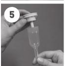
Snap the reservoir onto the insert.
